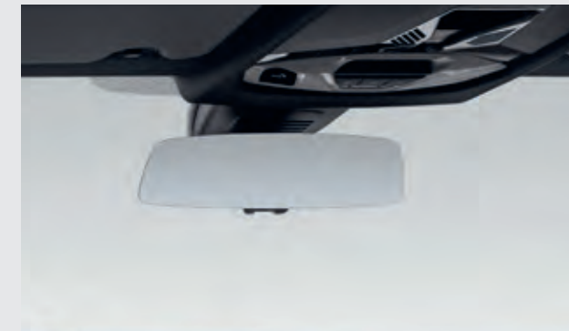
The Frameless Interior Mirror , with electromagnetic coating, consists of automatic anti-dazzle function via integrated sensors that measure light incident from behind and automatically dim the interior mirror if the measured light intensity is high enough to cause dazzling.
