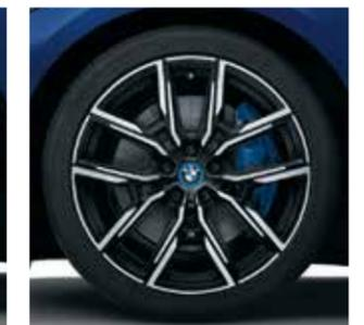
19" M light alloy wheels Y-spoke style 859 M Bicolour Jet Black uni with mixed tyres, gloss-lathed, wheel size front 8.5J x 19 with 245/40 R19 tyres, wheel size rear 9J x 19 with 255/40 R19 tyres.
