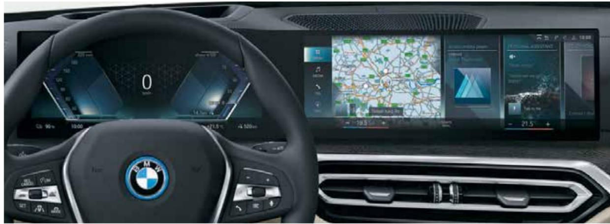
■ The BMW Live Cockpit Plus comprises a curved display combination with a 12.3" instrument display and a 14.9" control display with touch function.
