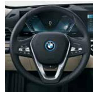
■ Servotronic steering continuously adjusts the steering effort required and steering force depending on the current speed and on the angle of the steering wheel.
