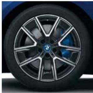
■ 18" M aerodynamic wheels 858 M Bicolour Black Grey with mixed tyres, gloss-lathed, wheel size front 8.5J x 18 with 245/45 R18 tyres, wheel size rear 9J x 18 with 255/45 R18 tyres.
