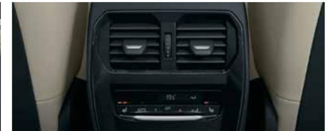
■ The Automatic air conditioning with 3-zone control and automatic temperature control features separate controls for you and your front passenger, as well as for the passengers in the rear. It also includes Automatic Air Recirculation (AAR), a micro active carbon filter, a fog and solar sensor, as well as rear air vents with a digital display.
