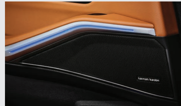
The tonally outstanding Harman Kardon Surround Sound System features a 464 W digital amplifier, nine channels and 16 speakers. Its sophisticated sound perfectly fills the interior space. Vehicle-specific, speed-dependent equalising precisely compensates for any background driving noise.
