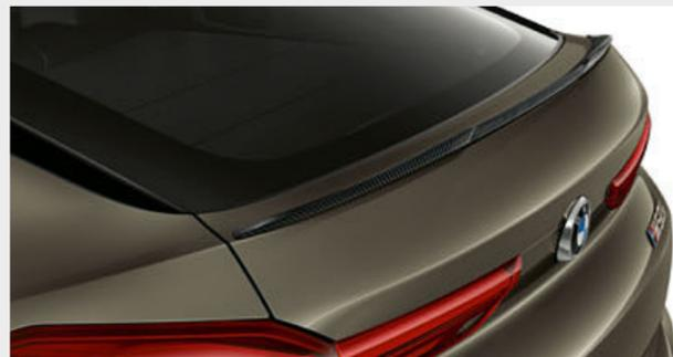
□ The M Carbon<sup>1,\*</sup> rear spoiler emphasises the vehicle's powerful, sporty design and noticeably reduces unwanted aerodynamic uplift on the rear axle.
