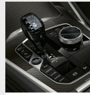
□ In the 'CraftedClarity' glass application, the gear selector, the iDrive Controller and the Start/ Stop button are made of hand-made crystal glass elements.
