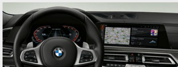
■ The BMW Live Cockpit Professional with navigation function<sup>3</sup> includes two high-quality displays network consisting of a high-resolution 12.3" Control Display that can be operated by touch and a fully digital 12.3" instrument display.
